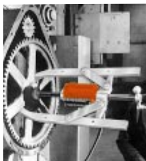
Power Team's hydraulically powered puller is shown removing a drive gear from an industrial shot-blasting machine.
