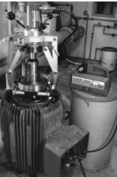
SGH153CR with a bearing pulling attachment was used to take a bearing off a utilities well pump motor.
