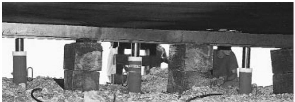
The newly constructed 256 ft. 1000 ton Branson Belle Showboat was launched into Table Rock Lake, MO. with the help of Power Team hydraulics. The hull was lifted using 10 Power Team C7513C 75 ton spring-return cylinders connected to a single manifold and powered by a PE553 electric pump.
