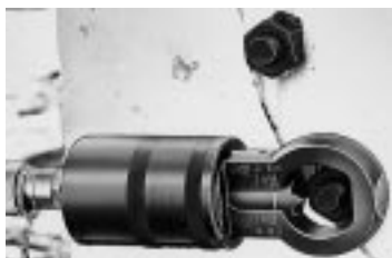
Align mark on cutter blade with scale.
