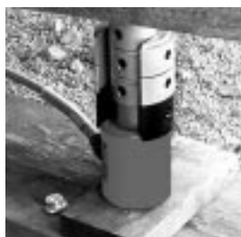
Cribbing blocks are shown here in use with a 30 ton RSS302 "Shorty" cylinder.
