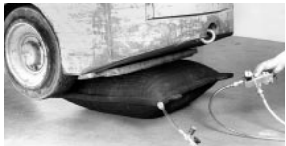
An Inflatable jack is shown lifting an industrial forklift, which has limited clearance for jacking.
