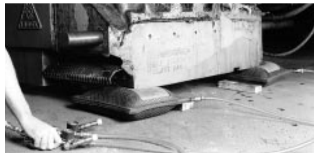
Moving machinery is a lot easier with inflatable jacks and their ability to handle off center loads and limited access.
