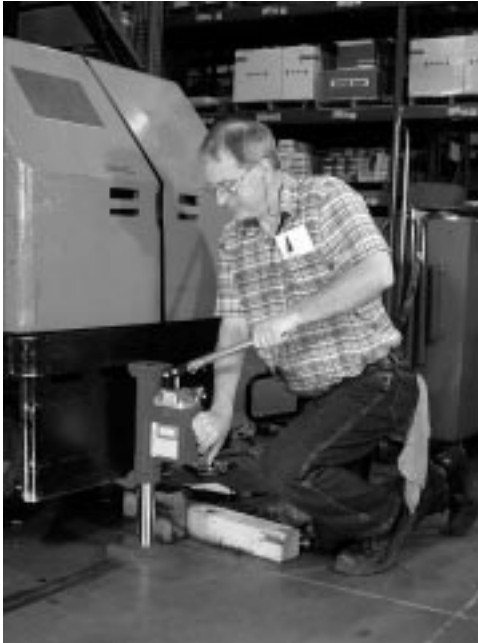
Lifting tasks having clearances as limited as one inch are easily performed with Power Team hydraulic toe-lift jacks.
